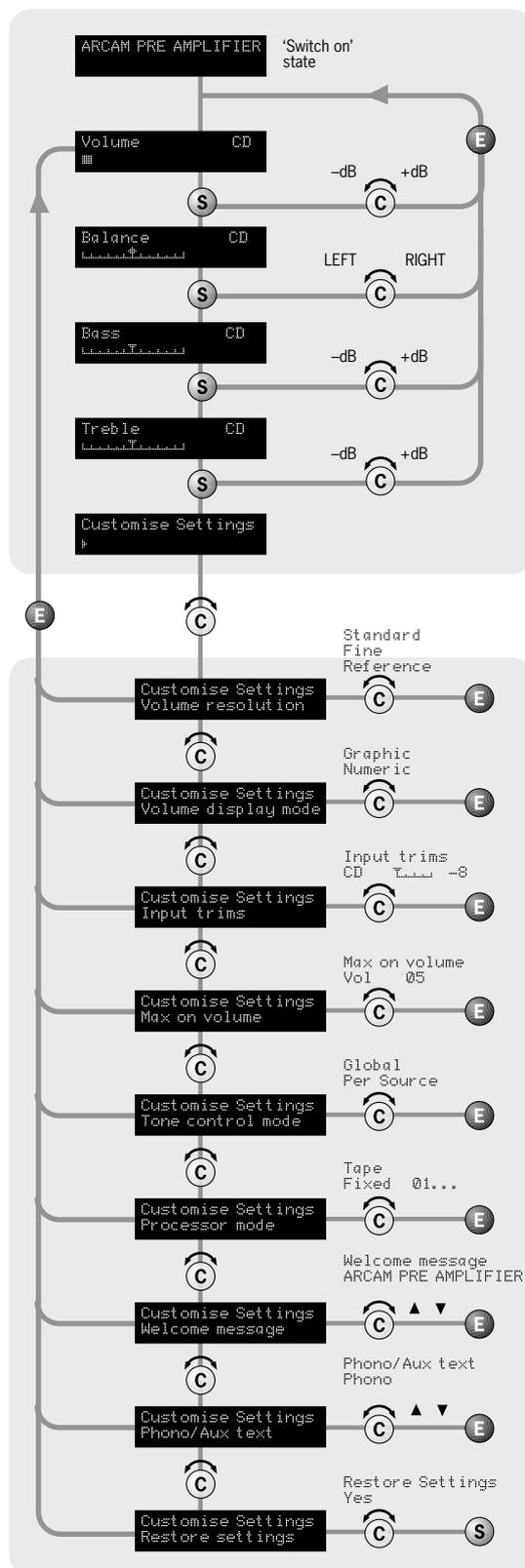
**Volume Resolution** – **STANDARD**, **FINE** or **REFERENCE**. 'Standard' and 'Fine' represent different levels of volume control sensitivity. The 'Reference' setting gives absolute increments in 0.5dB steps.
