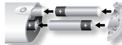
2. Insert four 'AAA' batteries into the battery compartment – two facing the top of the unit, and two facing the end, as in the diagram.
