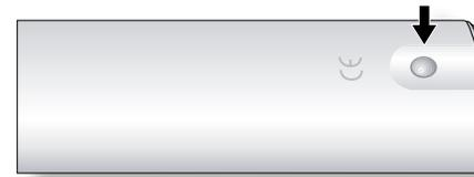
1. Open the battery compartment by pressing the button on the back of the handset.
