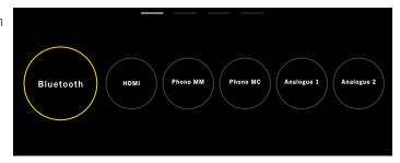
The Amplifier can recall 5 device pairings. If 5 are in memory already, the oldest will be replaced. Because portable devices have a volume slider with large volume steps, there is a maximum volume setting in the amplifier to prevent excessive volume output being selected accidentally. The default is 40.
