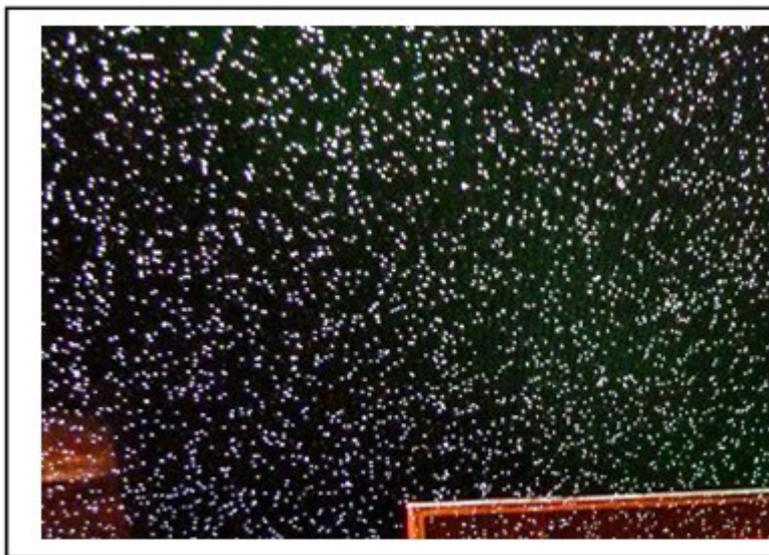
This is typically a problem caused by the cable either between the source component and AVR or most likely from the AVR to the Panel or PJ (the longer length)..
