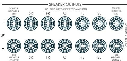
It is important that no stray strands of wire from these connections are allowed to touch another cable or the product casing. Failure to ensure this can cause a short circuit and damage your Receiver.
