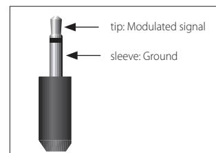
The infrared inputs (**Z1 IR** and **Z2 IR**) allow the connection of external IR receivers, either when the Receiver front panel IR receiver is fully or partially obstructed or to allow the use of a remote control in Zone 2.
