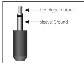
The trigger connectors (**TRIG Z1** and **TRIG Z2**) provide an electrical signal whenever the Receiver is switched on and the relevant zone enabled.
