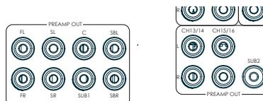
The Receiver also allows up to four active subwoofers to be connected to the **SUB** or **Ch13/14/15/16** outputs. Refer to your subwoofer handbook for the correct setting up and connection procedure for your particular subwoofer(s).
