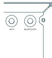
If using the Wi-Fi or Bluetooth features of the Receiver, please attach the single antenna for the Bluetooth and the two antennas for the Wi-Fi.
