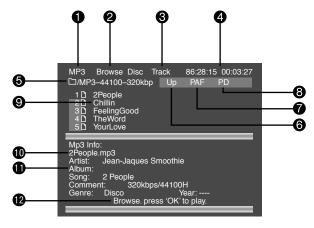
The screen shown above is the disc navigator screen, in this example showing a CD-R containing MP3 files. The following items can be identified:
