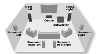
have a large 'hole' in the middle and will be presented in two halves. If there is no practical alternative to placing the speakers widely apart, this effect can be overcome in music reproduction by using centre sound extraction from the left and right speakers (see the description of 'Dolby Pro Logic IIx Music Mode' later in this handbook).
