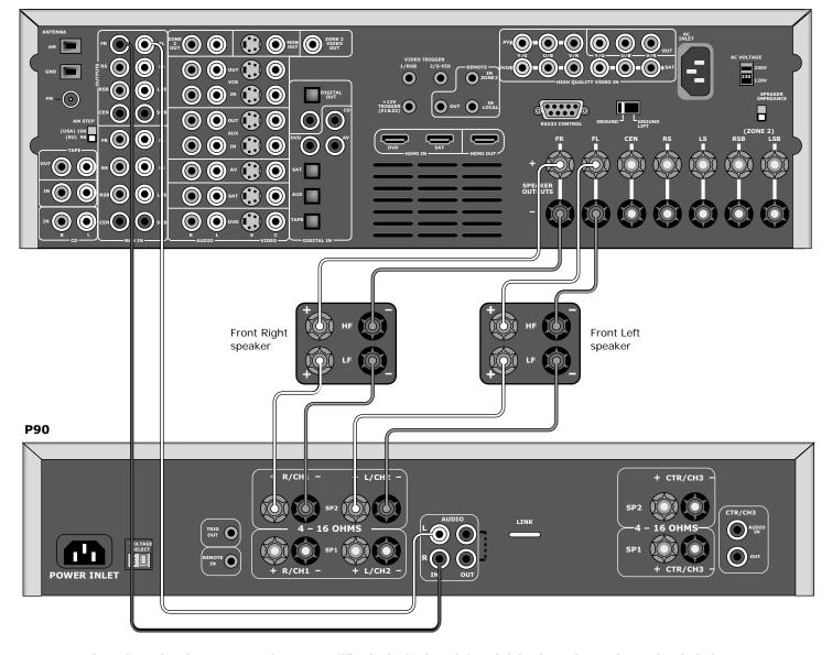
Bi-amping using the AVR350 and a P90 amplifier (only the front left and right channels are shown, for clarity)
