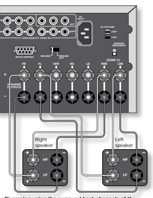
Bi-amping using the surround back channels of the AVR350 (only the front left and right speakers are shown, for clarity)
