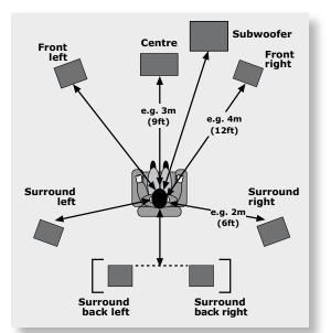
Distance measurements for 5.1 [and 7.1] speaker delay settings
