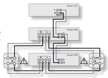
A P38 connected to speakers using bi-amping.
