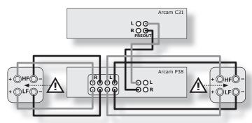
A P38 connected to speakers using bi-wiring.
