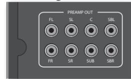
The AV950/AVR750/450/380 also allows an active subwoofer to be connected to the **SUB** output. Refer to your subwoofer handbook for the correct setting up and connection procedure for your particular subwoofer.
