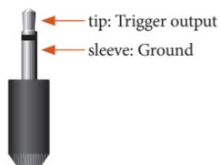
The trigger connectors (**TRIG Z1** and **TRIG Z2**) provide an electrical signal whenever the AV950/AVR750/450/380 is switched on and the relevant zone enabled.
