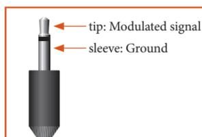
The infrared inputs (**Z1 IR** and **Z2 IR**) allow the connection of external IR receivers, either when the AV950/AVR750/450/380 front panel IR receiver is fully or partially obstructed or to allow the use of a remote control in Zone 2.
