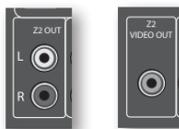
The Z2 out analogue audio connector can be used to connect the stereo audio output of the AV950/AVR750/450/380 to an amplifier located in a second room.
