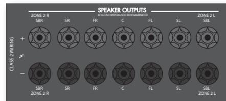
If the main zone has a 5.1-channel surround sound speaker system (not a 7.1-channel system), the spare SBL and SBR speaker outputs can be used to power speakers in Zone 2, so that a power amplifier is not required.
