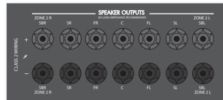
It is important that no stray strands of wire from these connections are allowed to touch another cable or the product casing. Failure to ensure this can cause a short circuit and damage your AVR750/450/380.
