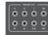
All preamplifier analogue outputs are buffered, have a low output impedance, are at line level and follow the Zone 1 volume control setting. They are able to drive long cables or several inputs in parallel if required.
