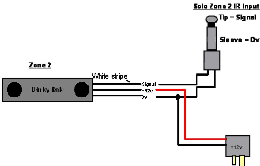
Solo also has the ability to provide a **+12v trigger** for control of ancillary devices such as power amplifier in the Second Zone; the +12v control is active when the Solo is not in Off or Standby modes.
