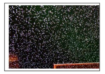
This is typically a problem caused by the cable either between the source component and AVR or most likely from the AVR to the Panel or PJ (the longer length).. Call up the set up menu on the AVR. Is this stable and free of noise? If so the length between the AVR and panel is o.k and the source to AVR link is suspect.. If noise is still present or picture disappears completely then the link between the AVR and Panel may be the culprit try an alternative brand or shorter cable..
